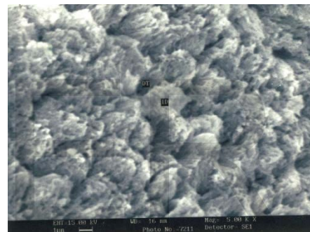
Fig-8-Dentin surface after acid conditioning without NaOCl wash.
